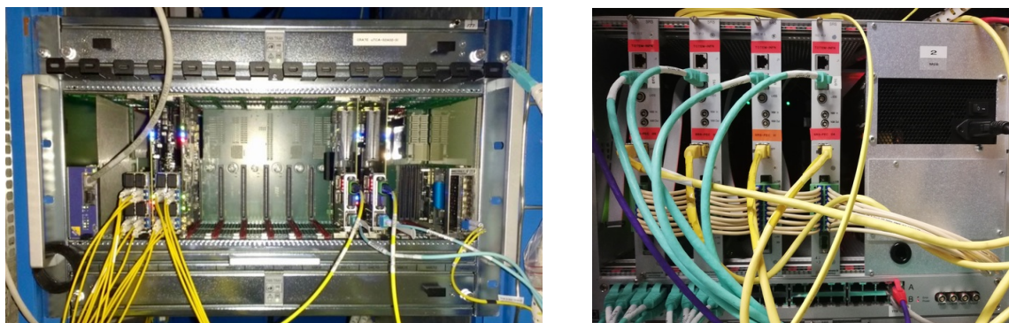
Figure 104. Left: the PPS pixel DAQ crate. On the left are two FC7 FECs, sending clock, trigger and slow-control commands; in the center-right are two FC7 FEDs, receiving data from the two arms of the PPS spectrometer; on the far left is the MCH crate controller, on the far right is the AMC13. Right: the timing and strips DAQ crate. The SLinks are placed in the backplane of the OptoRx boards delivering data to upstream CMS DAQ.
