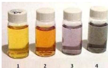
Fig. 3.2.1 Silver nanoparticle solutions with different sizes and concentrations. 1: 10 nm ( 3.6 \times 10^{12} Nps / mL), 2: 40 nm ( 5.7 \times 10^{10} Nps / mL), 3: 60 nm ( 1.7 \times 10^{10} Nps / mL) and 4: 100 nm ( 3.6 \times 10^9 Nps / mL).
