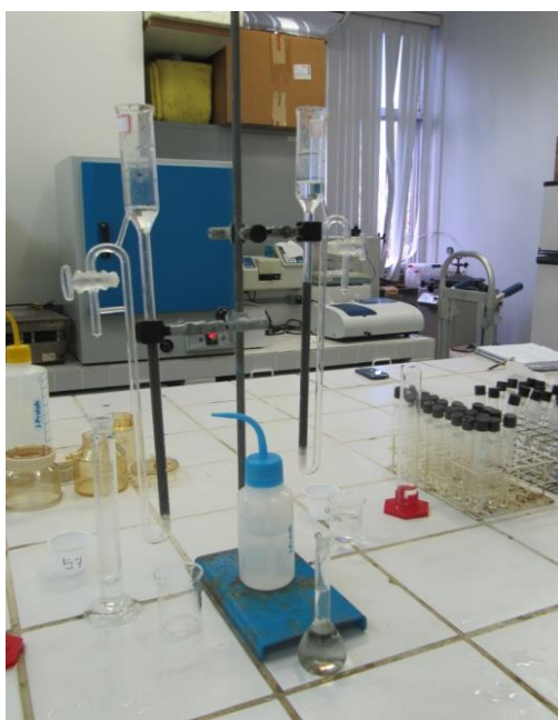
Figure 4.3. Cd column reduction method. Limnolab. (UFES)
