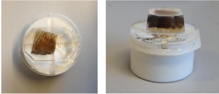
Figure 2.2: Embedded skin sub-samples in Technovit 7100. Blocks prepared for tissue sectioning with microtome.
