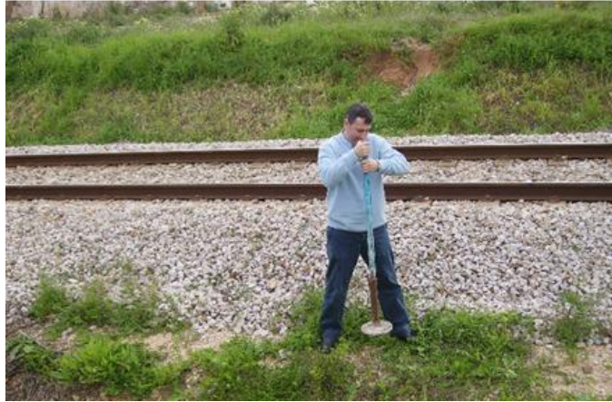
Figure 1 – Example of using mass to generate an impulse of vibration
