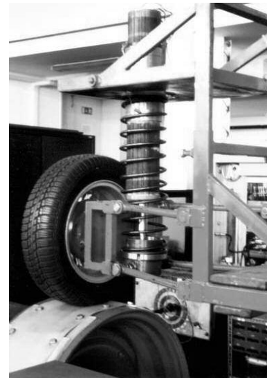
Fig. 13. Actuator prototype and partial view of the workbench.
