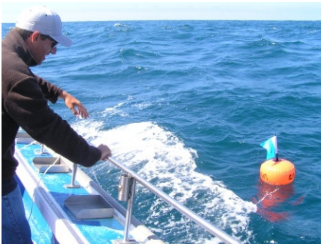
Fig. 2. Deployments of the autonomous receiver. Top panel: deployments for assisted operation from boat, and moored deployment; bottom panel: for assisted operation the hydrophone is allowed to drift away, in order minimize the noise of waves hitting the boat.
