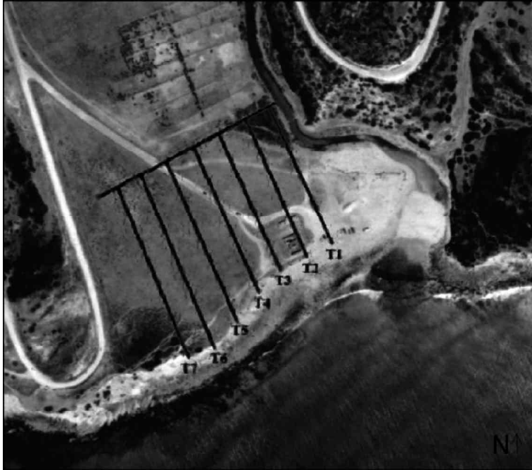
FIGURE 4. Aerial photo from 2001 showing the seven control lines normal to the coast and the imaginary shore-parallel line used to measure changes in the bluff position at Boca do Rio beach.
