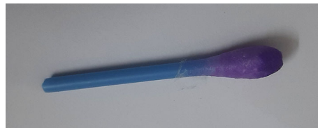
Figure 7. Violet colour indicates positive test for cadmium.
