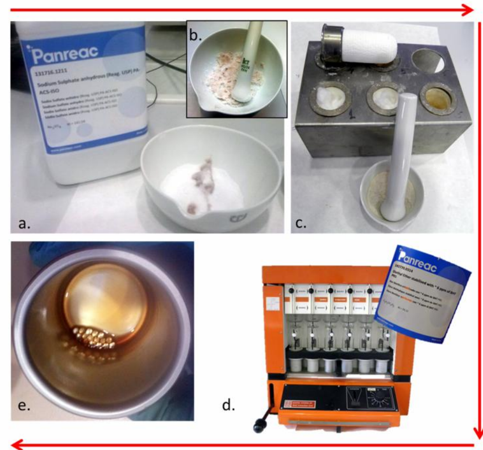
Figure 2.6.3. Crude lipid extraction by Method 920.39 (Cunniff, AOAC, 1997). a. and b. - moisture extraction; c. - capsules for lipid extraction; d. - SOXTEC AVANTI 2058; e. - extracted crude lipid.
