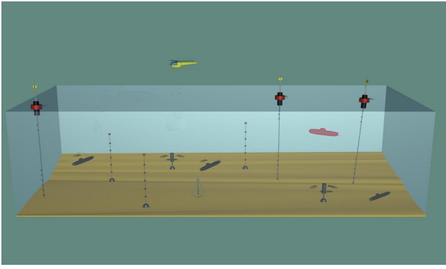
Fig. 2. Mobile communication network involves the integration of acoustic and non-acoustic systems for collecting and mobile nodes for uploading environmental information
