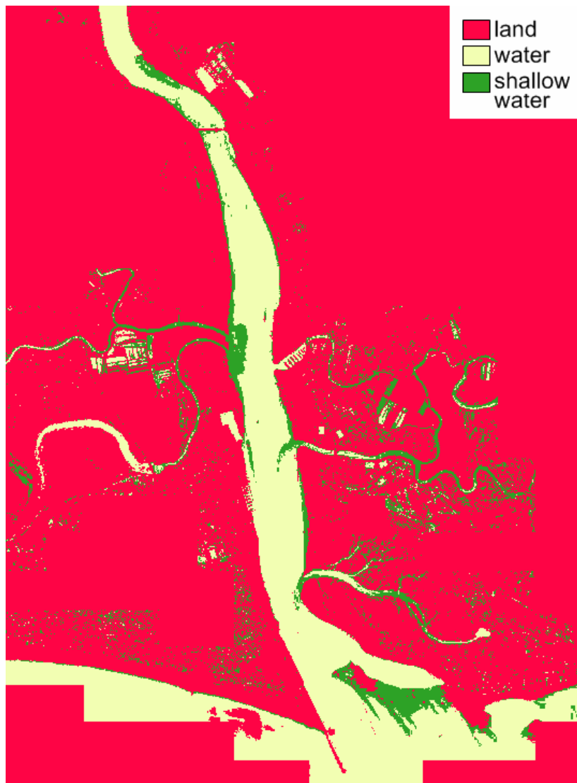
Figure 4.14. The final PCA-based classification result.
