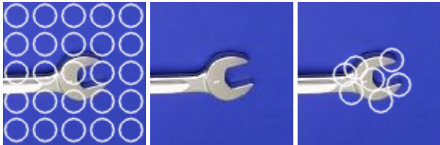
Fig. 2. Data selection step. Center: image from Caltech 101. Left: keypoints sampled from a regular grid. Right: our keypoints. Only one scale is shown for clarity.
