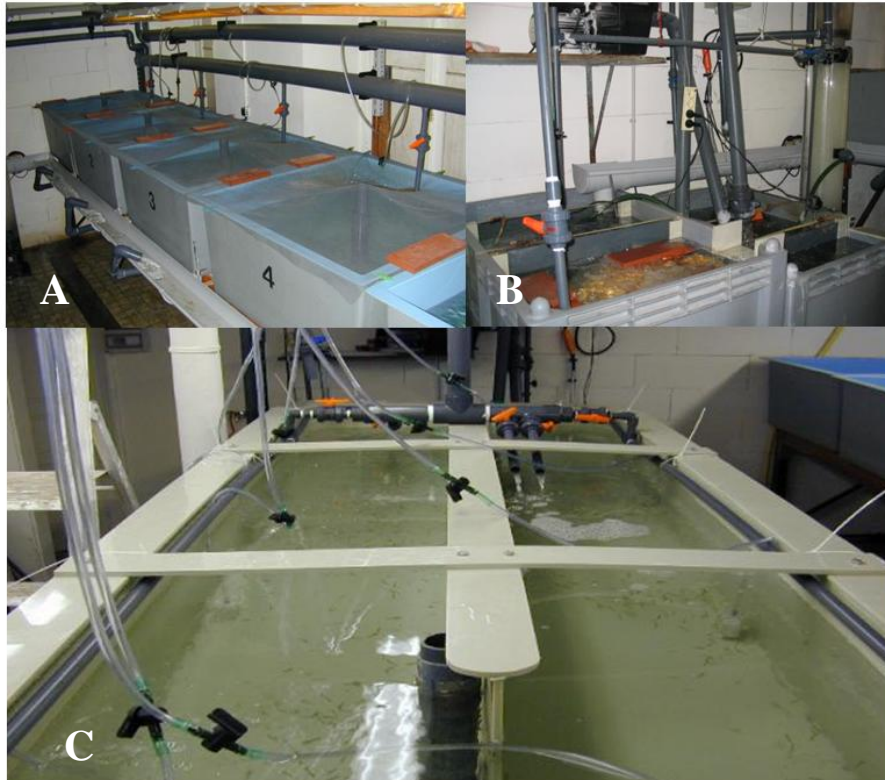
Fig. 13 – Recirculation system for raising shrimp at the the facilities of the Laboratory of Aquaculture and Artemia Reference Center. A – 250L tanks; B – Biological filter; C – 3000L raceway-tank
