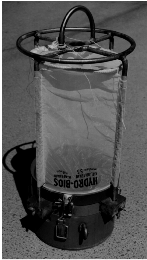
Fig. 3 – Cylindrical net container with 25 cm diameter and 50 cm high, used for calibration of RNA/DNA ratio of sardine larvae. There were two types of containers: one with mesh size of 10 mm which did not allow the entrance of sardine prey and the other with mesh size of 500 mm through which food organisms could pass.
