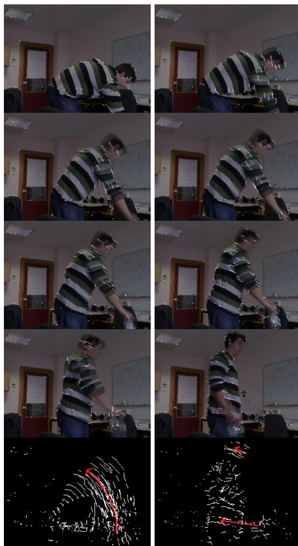
Fig. 4. The optical flow model applied to a person after fetching a bottle from the floor. The sequence shows vectors between successive frames. The two bottom images show the combined vectors while straightening (left), followed by bringing the arm and bottle close to the body and moving the head (right). Significant motions attributed to tracked, segregated regions are indicated by the red arrows.
