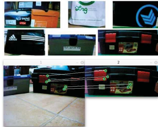
Figure 3: Top two rows: examples of learned objects. Bottom: example of object recognition with 5 matching keypoints.
