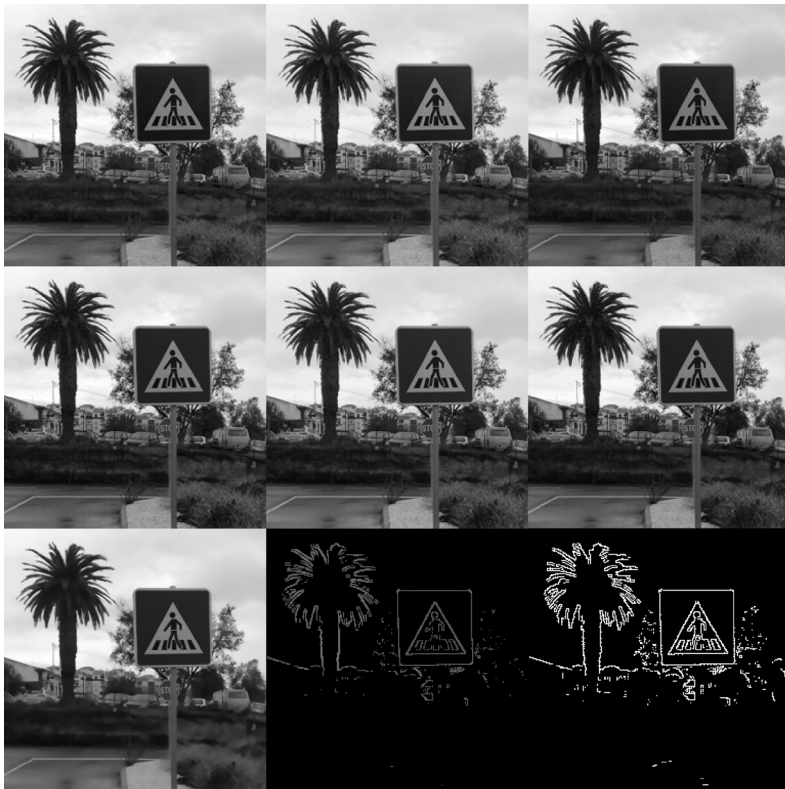
Fig. 3. Top and middle: colour illuminant and geometry normalisation; input images (top) and respective results (middle). Bottom, left to right: adaptive colour-region filtering, border saliency by colour conspicuity, and non-maximum suppression.
