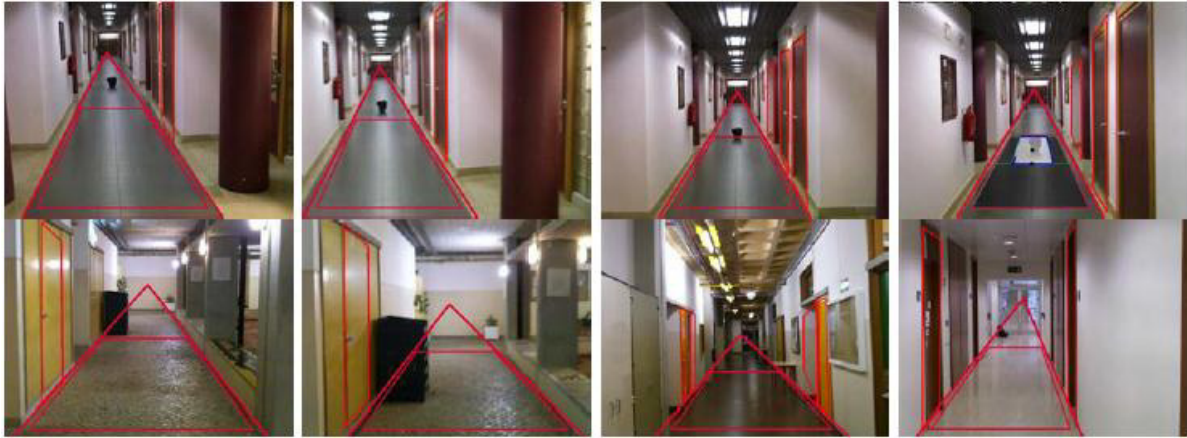
Fig. 2. Top: path, obstacle and doors detected along a corridor. Bottom: more examples in other corridors.
