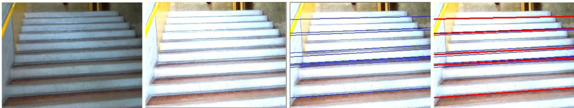
Fig. 4. Left to right: example image with stairs, brightening and sharpening, detected horizontal edges and final steps detected.
