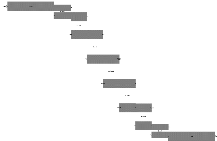
Figure 6.18 - Layout of the bandpass filter with f_c=9\text{ GHz}
