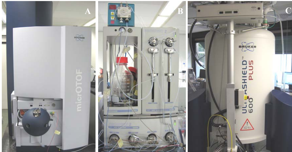
Figure 3.2.1 - Equipment used for the HPLC-ESI-MS and HPLC-SPE-NMR experiments: Bruker Daltonics microTOF (time of flight) ESI mass spectrometer (A), Spark Holland Prospekt 2 SPE unit (B) and Bruker Avance III 600 MHz NMR spectrometer (C).
