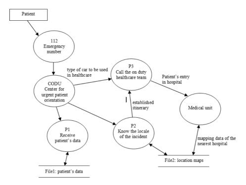
**Figure 1**. Diagram of data flows and main processes in INEM's information system (source: interview with an INEM executive)
