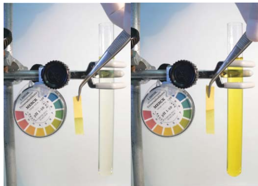
Fig. 3 Photography of two vanadate solutions, at ambient temperature, obtained from a 10 mM metavanadate solution, pH 6.8, before (left) and after addition of HCl (final pH of 6.6 (right)). Decavanadate solutions correspond to the latter situation, after the pH value is ascertained, to a final pH of 4.0. Vanadate solutions were prepared from solid \text{NH}_4\text{VO}_3 . The addition of conc. HCl induces the formation of decameric vanadate species responsible for the yellow colour of the solution (adapted from ref. 15).
