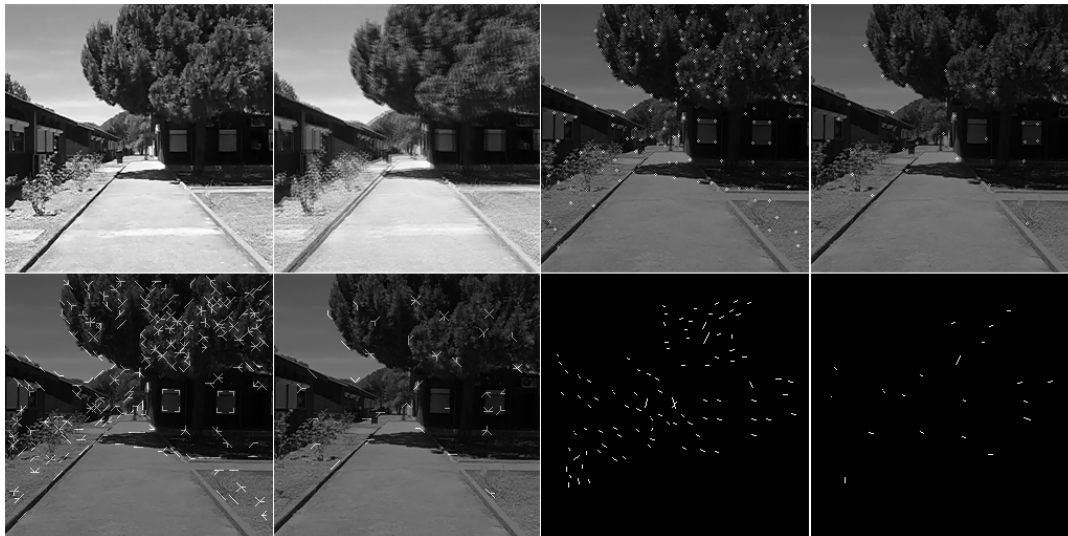
Figure 7. Keypoint detection, annotation and matching. Top, from left: one frame of the sequence shown in Fig. 4, two successive frames combined, and detected keypoints at scales \lambda = 6 and 15. The bottom row shows annotated keypoints and displacement vectors between the successive frames at the two scales.
