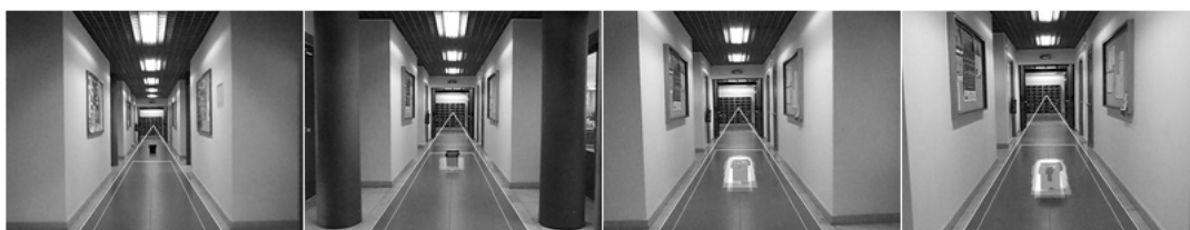
Figure 6. A sequence with detected path borders, the obstacle detection window, and a looming obstacle which has been detected.
