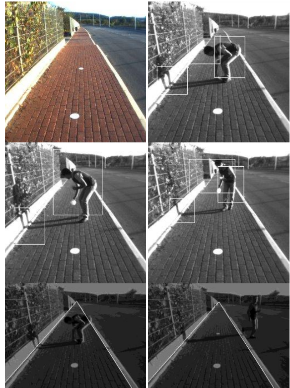
Figure 4. Top-left: input frame with markers. Top-right and middle: a moving person is picking up one marker and has been detected, also the person's shadow (white rectangles). Bottom: detected sidewalk borders with and without partial occlusion.
