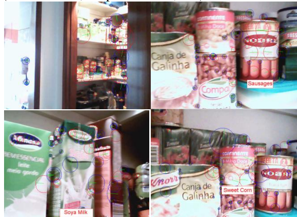
Figure 5. Typical views of household items on shelves which have been located and recognised using the OpenSURF software.
