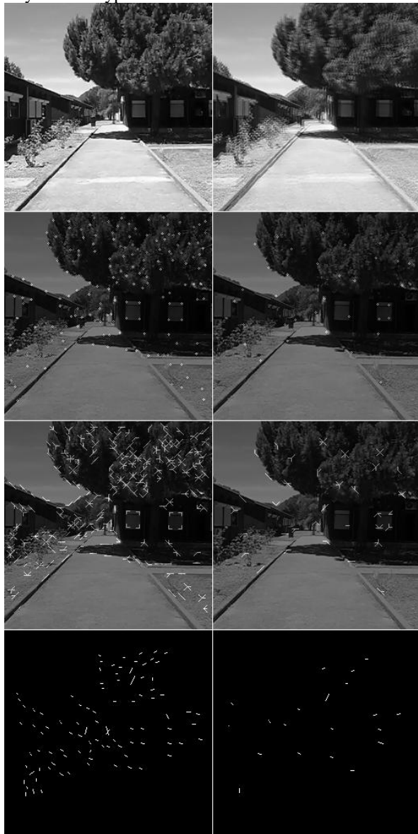
Figure 6. Keypoint annotation and matching. Top: one frame from the sequence shown in Fig. 1 (left) and two successive frames combined (right). The second row shows detected keypoints at scales \lambda = 6 (left) and 15 (right). The third row shows annotated keypoints and the bottom row displacement vectors between the successive frames (top-right).
