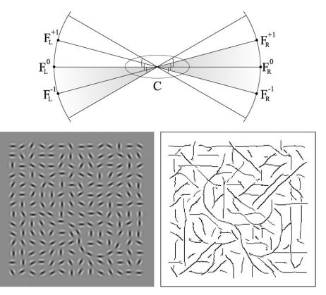
**Fig. 4.** Top: continuity processing with center- and fan-summation areas, *C* and *F*, in case of horizontal events with curvature (see text). The shading shows combination  $F_L^{-1} - C - F_R^0$ . Bottom-left: test image with Gabor patches and "snakes" embedded in randomized patches. Bottom-right: detection result.
