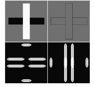
**Fig. 1.** Input pattern (top-left), the summation of lateral and cross-orientation inhibition for  $\theta = \{0, \pi/2\}$  (bottom) and the detection result (top-right) with no spurious events beyond the corners and no gaps at the junctions.
