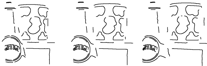
Fig. 8. Three view matching. 25 contour chains are matched. There is only one incorrect match which arises from a specularity on the bottle.
