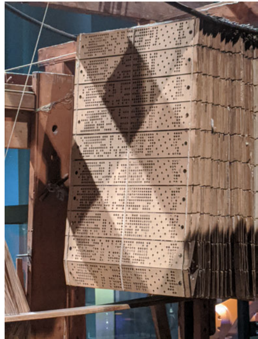
(b) The punch cards used in the Jacquard loom for a programmable pattern—each row of punched holes in these cards corresponds to a row of the textile being woven
