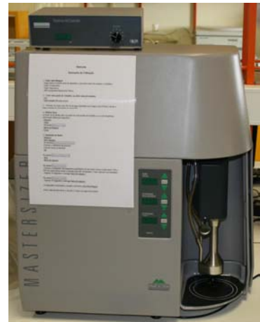
Figura 7.7 Malvern Mastersizer na FCMA (UAlg).
