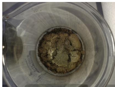
Figure 8: once realized charring at 500 °C
