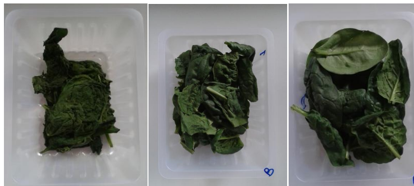
Figure 34 – Samples of spinach without packaging, packed with TPS-based film and packed with PVC film (from left to right respectively), at day 7
