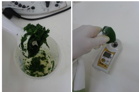
Figure 18 - Preparation of the sample (left) and brix measurement on the refractometer (right)
