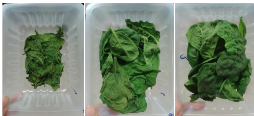
Figure 36 – Samples of spinach without packaging, packed with TPS-based film and packed with PVC film (from left to right respectively), at day 11
