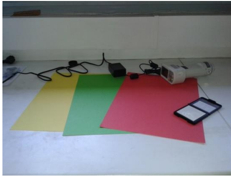
Figure 13 – Colorimeter, white tile and yellow, green and red cardboards
