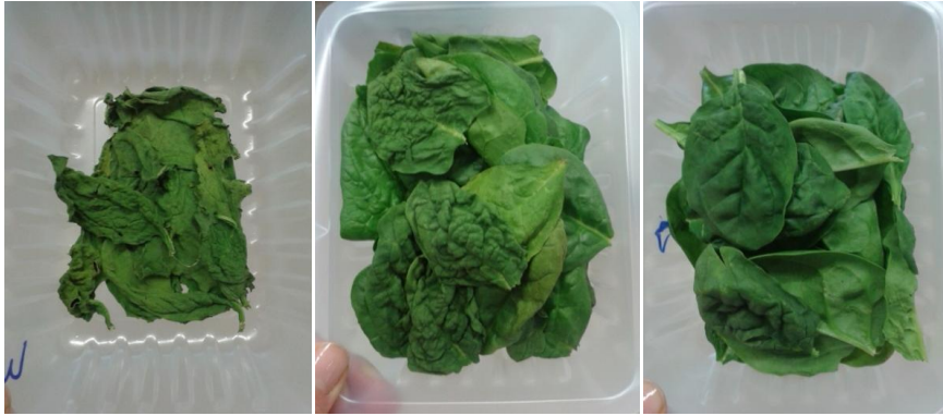
Figure 37 – Samples of spinach without packaging, packed with TPS-based film and packed with PVC film (from left to right respectively), at day 14
