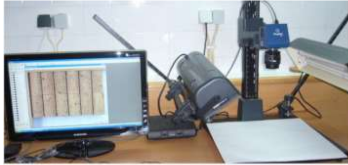
Figure 15. Image analysis system used for the surface observation of cork stoppers.
