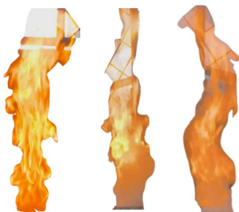
Fig. 7. Flame color from burning biomass with fuel with drying temperature (a) 70 °C (b) 90 °C (c) 110 °C.
