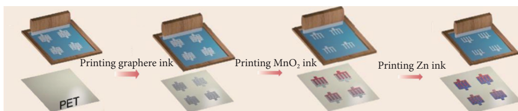
Figure 4 Schematic diagram of screen printing manufacturing of printed Zn/MnO 2 MBs. Reprinted with permission from Ref. [31], © 2019 The Author(s).
