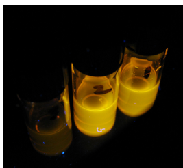
Figure 8. Luminescence of 5 \mu\text{M} CdSe QDs in toluene in the presence of (from left to right): carboxylic acid nitroxide 3 (2500:1 moles of nitroxide 3 :QDs), TEMPO (2500:1 moles of TEMPO:QDs), and no additive upon illumination with a TLC lamp at 366 nm.
