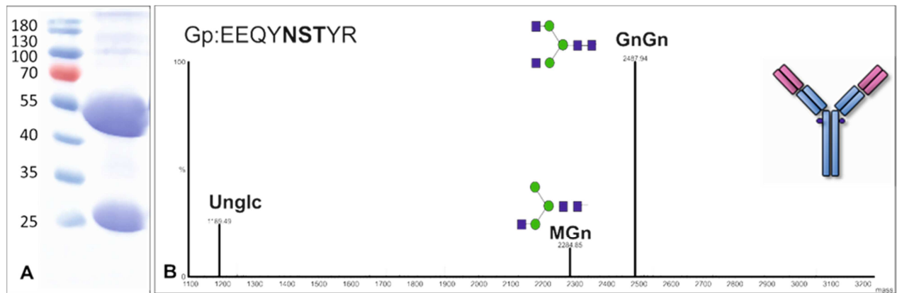
Figure 12: Small scale purification and glycan analysis of Rituximab expressed in N. benthamiana \Delta XF plants. (A) SDS-PAGE followed by Coomassie Brilliant Blue staining of reduced sample shows two bands of ~55 and 25 KDa corresponding to the heavy and light chain respectively. (B) N-glycosylation profiling by LC-ESI-MS of tryptic Fc glycopeptide (EEQYNSTYR) confirms a great majority of the antibody decorated with the targeted GnGn glycoform. Peaks were labelled in accordance with the ProGlycAn system ( www.proglycan.com ). Schematic representations of N-glycans structures detected are also shown. Plant material was then used for large scale purification and quantification.
