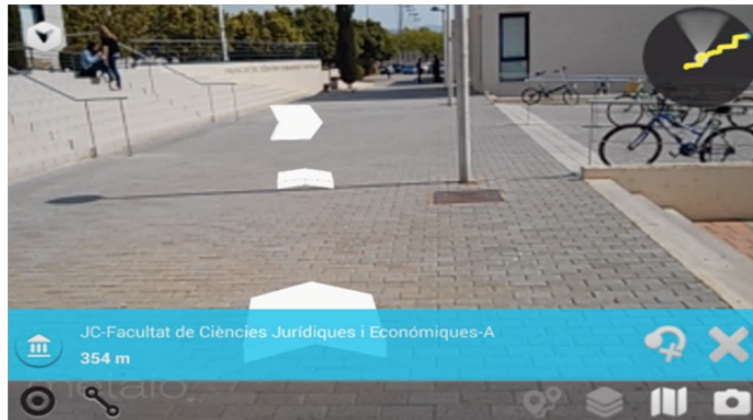
Fig. 3. Screenshot of the augmented reality application. It shows the path that the user should follow to reach its destination with white arrows.
