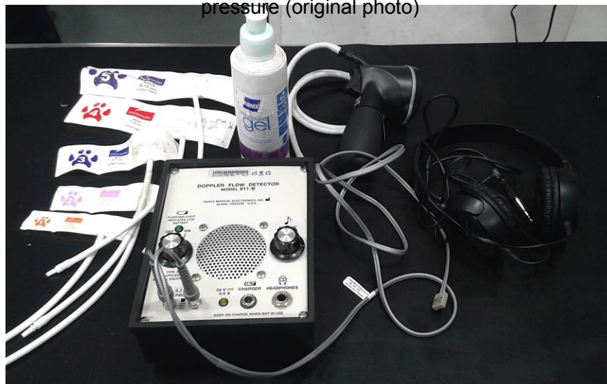
Figure 13 – Doppler Ultrasonography equipment used in the measurement of systolic blood pressure (original photo)
