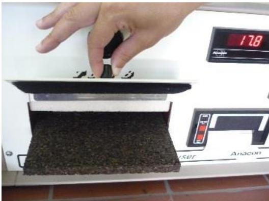
Figura 28: Thermal Conductivity Analyser
