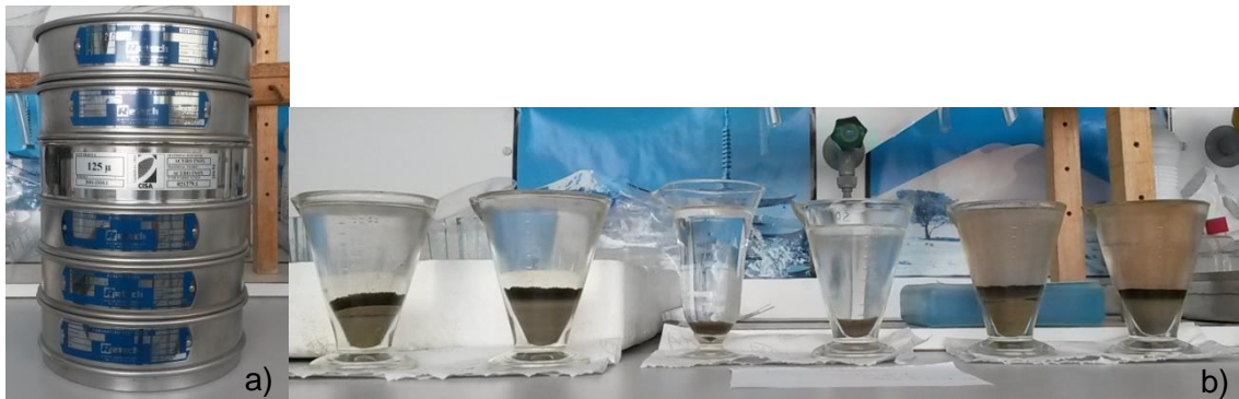
Figure 16 - Sieving and CSF technique: a) sieves used; b) sedimentation glasses with the sieved samples (original)
