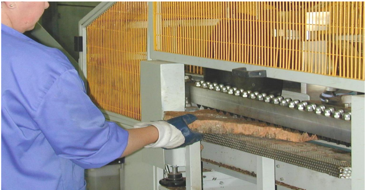
Figure 12. Cutting cork strips with automatic functioning
