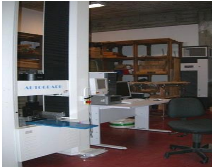
Figure 24. Universal test machine, equipment for mechanical tests of materials
