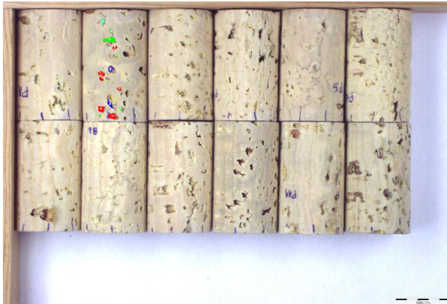
Figure 23. Frame with the stoppers, tresholding and detecting the pores in the second stopper
