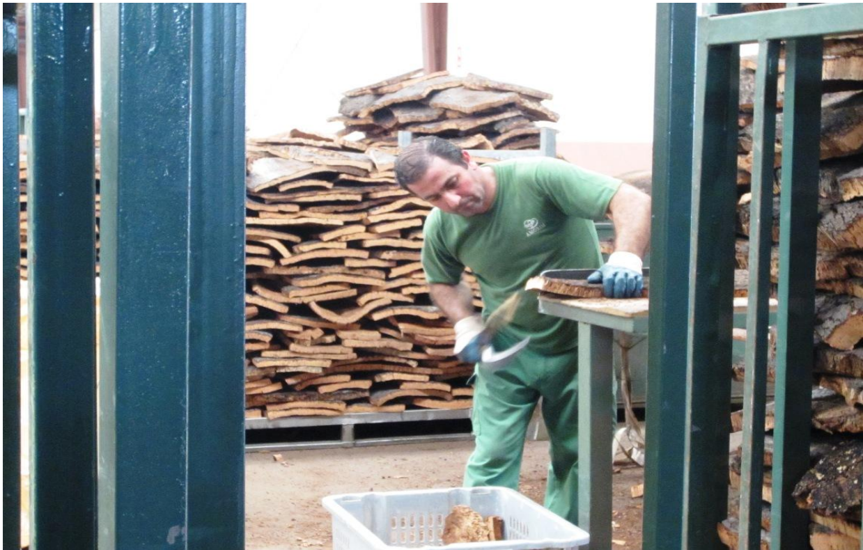
Figure 11. Trimming of the edge of the plank
