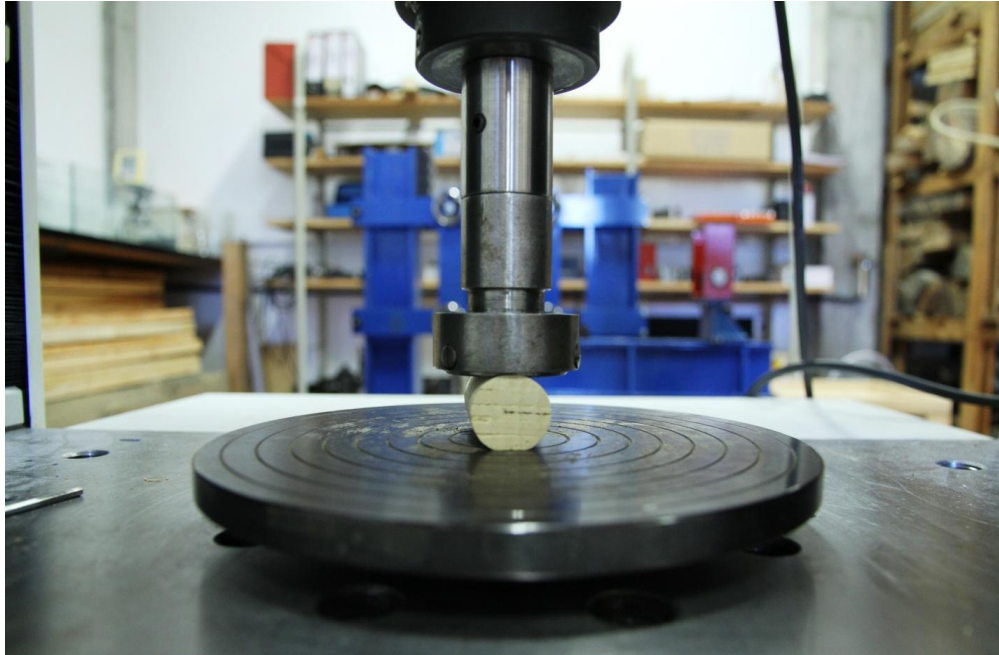
Figure 25. Transversal ompression test conducted on cork body surface
