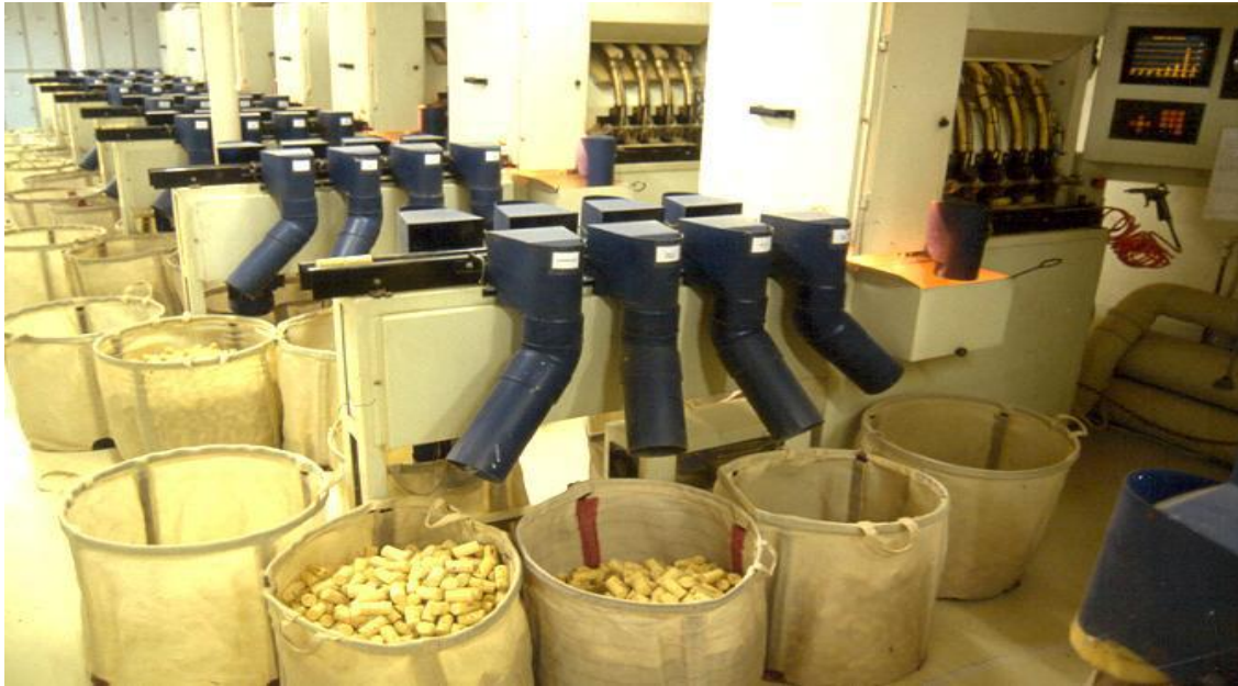
Figure 14. Automatic sorting machine based on vision technics
