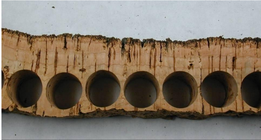
Figure 13. Cork strip after punching out a stoppers using automated equipment
