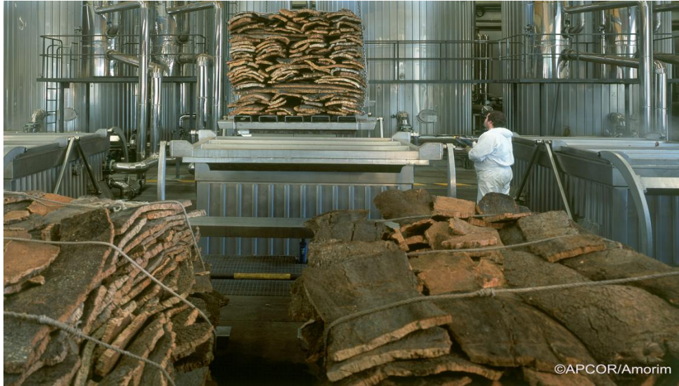
Figure 10. Boiling operation of planks in closed autoclaves: placing pallet with cork planks in the autoclave
