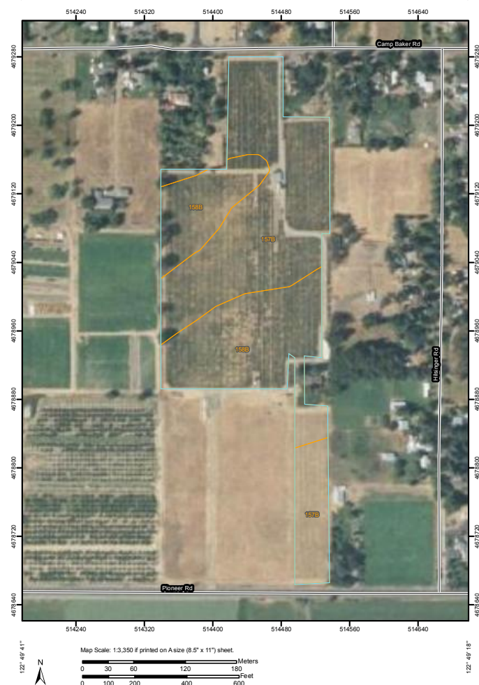
Figure 7. Soil survey map of Site 1. Soil types are indicated by the following codes: 157B) “Ruch silt loam, 2 to 7 percent slopes”; 158B) “Ruch gravelly silt loam, 2 to 7 percent slopes”. Provided by the United States Department of Agriculture, NRCS ( http://websoilsurvey.nrcs.usda.gov ). Exact soil borders may not be reliable to this scale.
