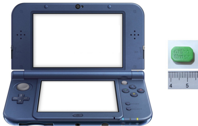
Figure 1 The handheld dichoptic games console used to administer the balanced binocular viewing treatment (left) and temperature sensor/logger with centimetre scale used as occlusion dose monitor for patching treatments (right).
