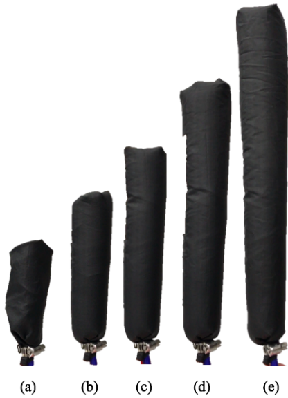
Fig. 3. Fabric-based eversion finger growing from the tip when inflated: (a) initial state of the fabric-based eversion finger when no input is given and the finger is in a folded state; (b-d) pressure input causes the finger to start growing from the tip by turning out its folds; (e) the finger is fully everted and achieves its maximum length [23].
