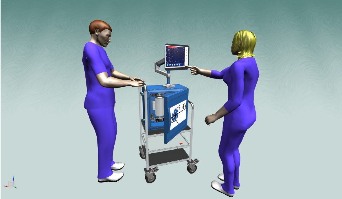
Figure 2: Preliminary CAD model of the HEV proposed design. The overall dimensions can be seen, together with the placement of the major components in the HEV cabinet.
