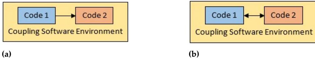
**Figure 5.1.** (a) One-way coupling and (b) two-way coupling.
