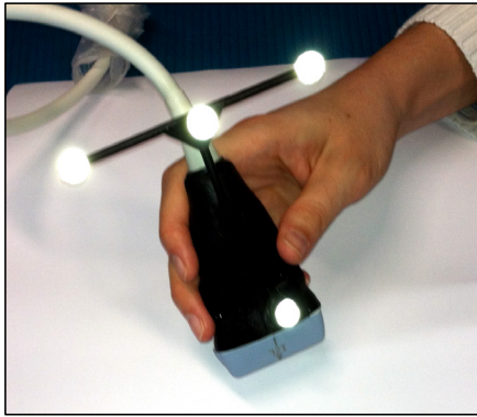
Fig. IV-3. Ultrasound transducer with a customized cluster composed by 4 non-collinear reflective markers fixed to the long axis of the transducer.
