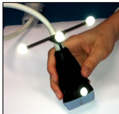
Fig. I-3. Ultrasound transducer with a customized cluster composed by 4 non-collinear reflective markers fixed to the long axis of the transducer.
