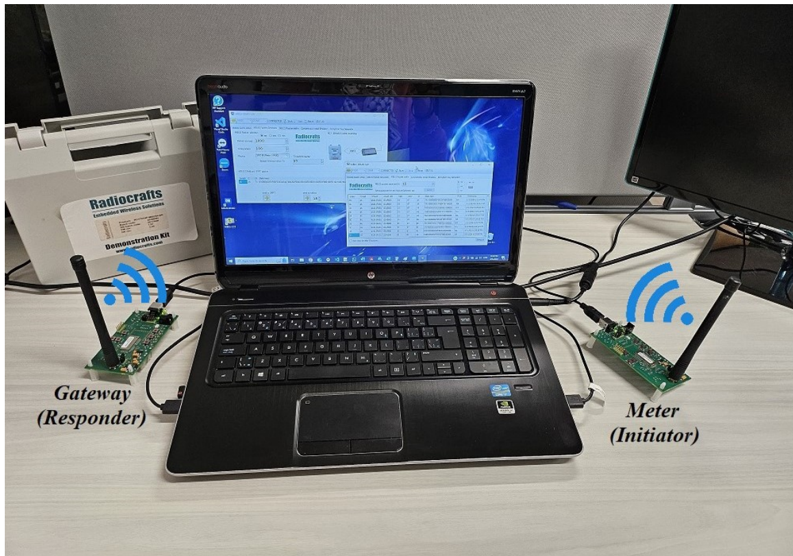
Figure 4.5: A wM-Bus communication setup with a laptop connected to a Gateway (Responder), and a Meter (Initiator), part of a Radiocrafts demonstration kit.
